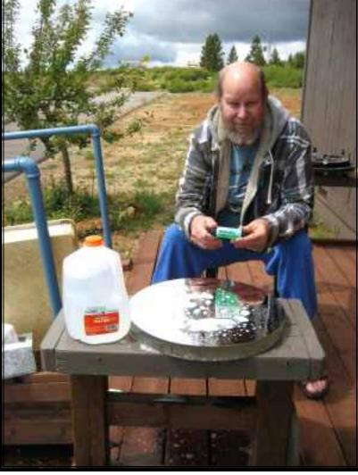
mirror cells are designed, and this one is bit different. It's very functional incorporating a standard nine point wiffle tree flotation sitting on crown nuts, but notice how the mirror edge is supported and secured. There are four clips with
